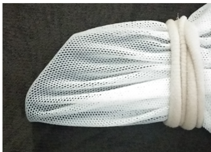
Figure 3: Nozzle protected with a tulle fabric. Image by the author.
