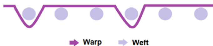
Figure 1: Weft and warp cutting section. Diagram by the author.
