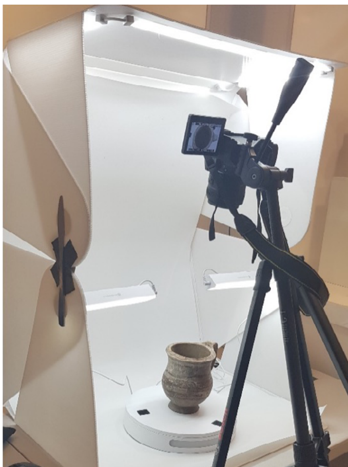
Figure 5: The camera, lightbox and turntable set-up.
