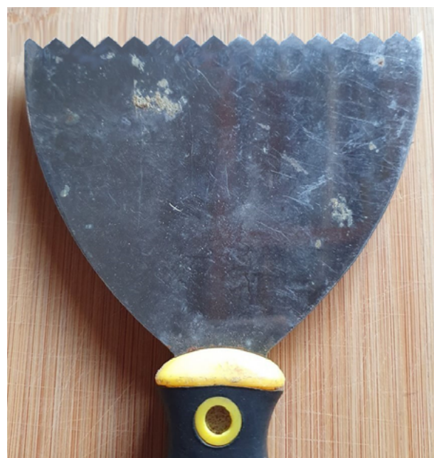
Figure 1: 21 st century toothed spatula customised to imitate the design of those used for the Florentine method. Photograph taken by the author.
