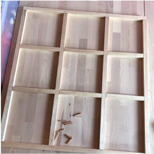
Figure 2: A wooden lattice, pine wood 600 x 600 x 18 mm with wooden dowel pin joints. Image by the author.
